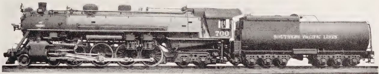
One of Fourteen 4-8-4 Type Passenger Locomotives, Built for the Southern Pacific Lines by The Baldwin Locomotive Works in 1930
